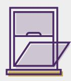
*Easy-to-Open Sashes on Double-Hung Windows:* Low-profile latches on the meeting rail release the sash to tilt in. This allows for interior and exterior cleaning to be done from the inside of your home.
